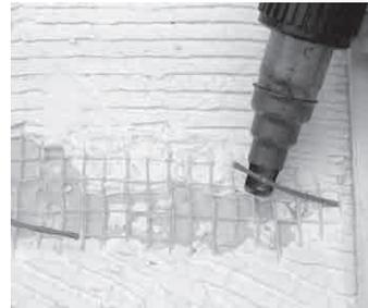
**Step 4.4.** With either type of jacket, if the jacket slug doesn't easily pull off you may need to use your heat gun to gently warm the slug, which should soften and loosen it for you. Use the heat gun (set to about 500°F) and move the gun back and forth under the jacket slug for about 3 or 4 seconds, or until it can be easily removed.
