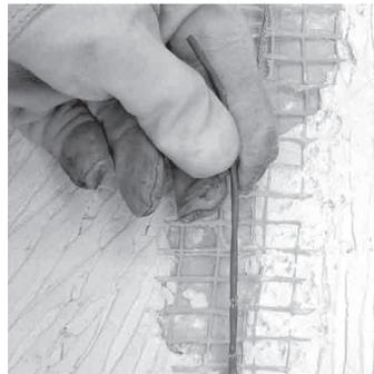
**Step 3.5.** Use a glove or other protective cloth to pull off the loosened jacket slug. **Do not touch** the hot jacket slug with bare fingers. The slug will be very hot and will burn!
